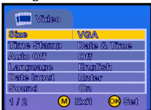
Using the **VOL-** button, scroll down to: Date input - Enter
