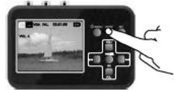
3. Select the desired recording using **◀◀** or **▶▶** buttons.
