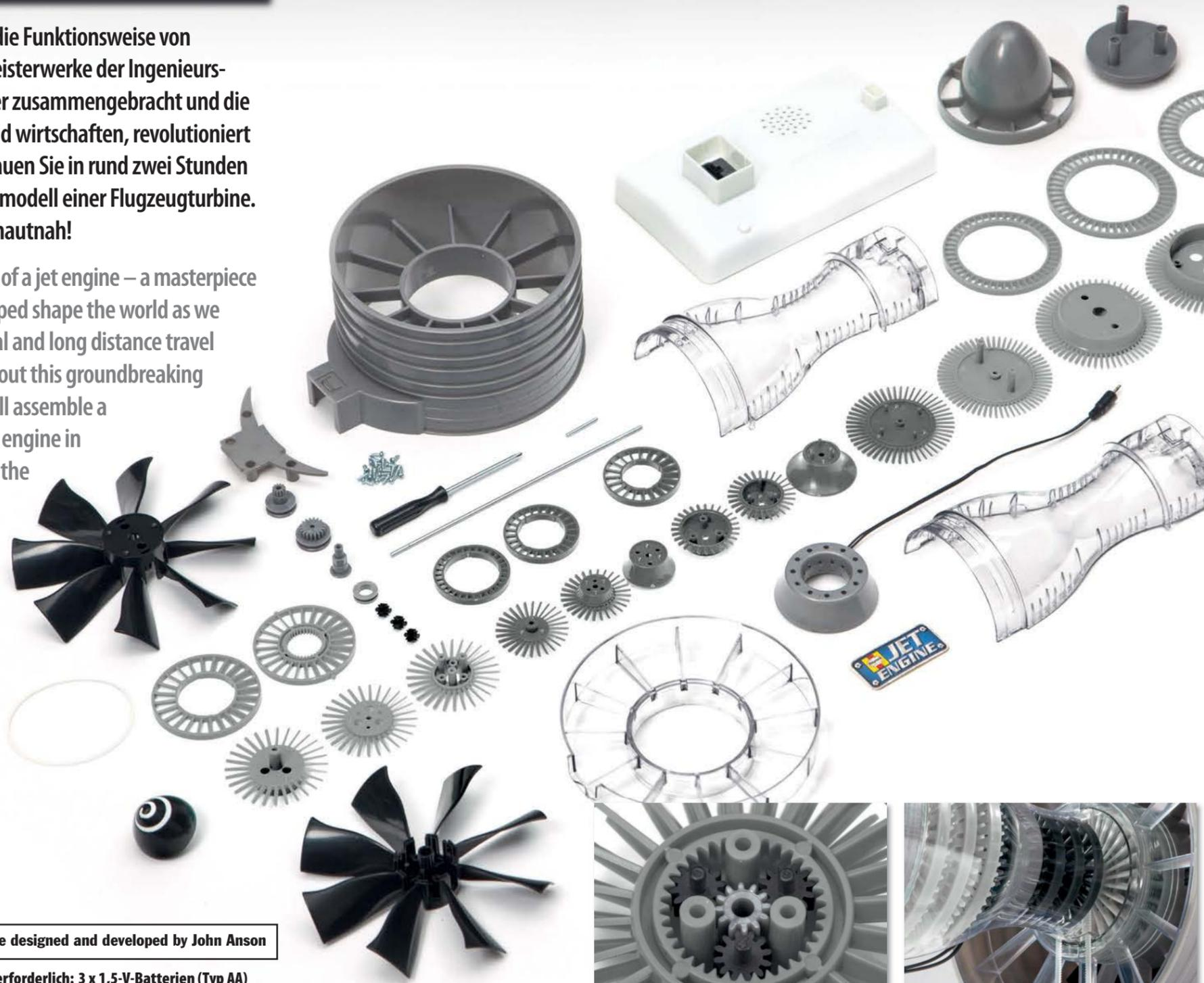
Jet engine designed and developed by John Anson
